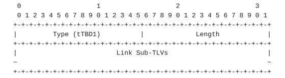
A link TLV describes a single link. It comprises a number of link sub-TLVs for the information described in section 4, which are the sub-TLVs defined in RFC 3630 or their equivalents except for the local IP address with mask length defined below.
