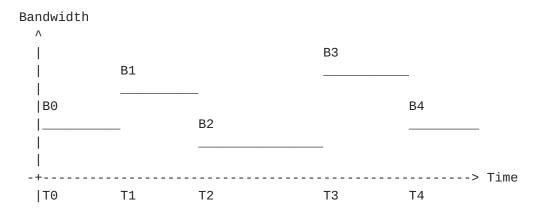
If an LSP is completely deleted at time T and uses bandwidth B, then for every time interval/period (after time T) during which bandwidth B is reserved for the LSP on a link, B is added to the link for that interval/period.
