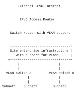
Figure 1: IPv6 deployment using VLANs (physical diagram)
