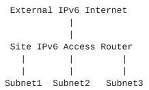
Figure 2: IPv6 view of the deployment (logical view)
