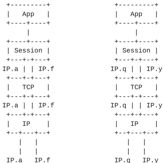
The problem with this approach is that a full session layer typically replicates substantial portions of the transport service, in order to ensure reliability and in-order data sequencing. This makes the session-level approach notably complicated and inefficient.
