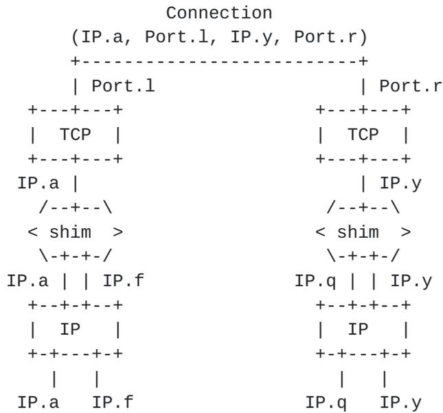
The transport layer is presented with the same service -- including the same apparent "addressing" model -- as previously. However the address is actually used as an identifier that maps to a set of locators. In the shim model, the identifier may be one of the valid locators.
