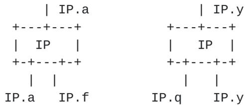
This example shows each host being multihomed. However a given association must choose a single IP Addresses, at each end, and bind the connection to it.
