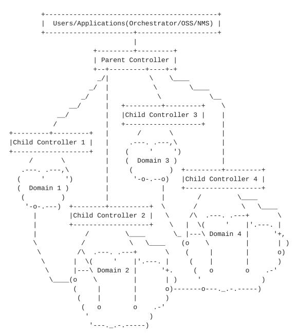
The parent controller communicates with these four child controllers and controls them, each of which controls (or is responsible for) a domain. Child controller 1 controls domain 1, Child controller 2
