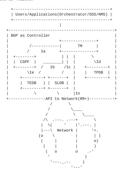
o Interface Ia between the TM and the CSPF. Through this interface, the TM requests the CSPF to compute a path for a tunnel with a set of constraints, and the CSPF responses the TM with the path computed that satisfies the constraints.
