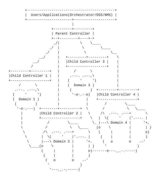
The parent controller communicates with these four child controllers and controls them, each of which controls (or is responsible for) a domain. Child controller 1 controls domain 1, Child controller 2 controls domain 2, Child controller 3 controls domain 3, and Child controller 4 controls domain 4.
