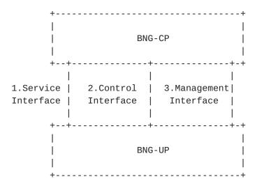
Internal interfaces between the CP and UP of the BNG device
