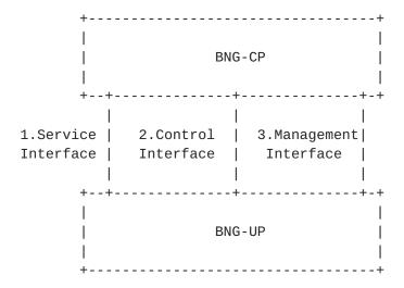
Internal interfaces between the CP and UP of the BNG device
