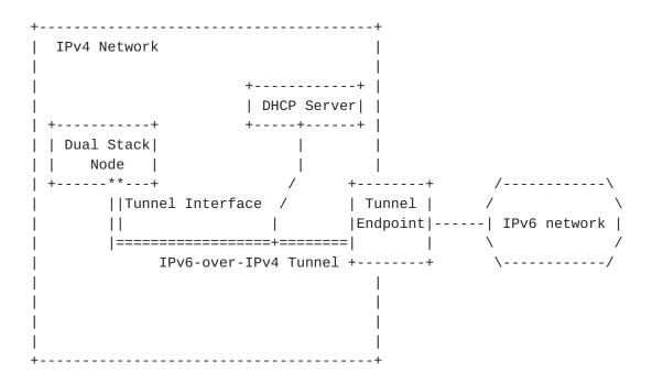
Fig. 1, Simple network model for TEP option use case
