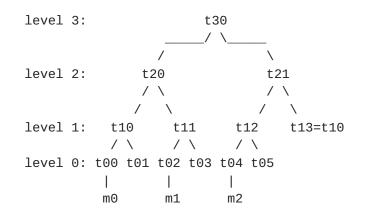
In general, let n be the number of input messages. If n is greater than  $2^31$ , the signing procedure fails and returns an error. Otherwise, it builds a tree with 1 levels numbered 0 to 1-1, where 1 is ceil(log\_2(n)) + 2. Hashes in the tree are built from the following functions:
