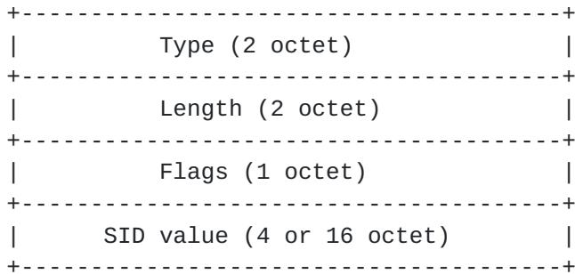
Figure 1: Segment Identifier(SID) TLV
