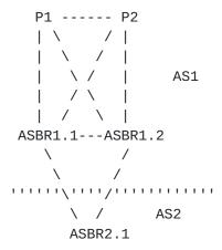
When the session between ASBR1.1 and ASBR2.1 undergoes maintenance, it is required that all i-BGP peers of ASBR1.1 reroute traffic to ASBR1.2 before the session between ASBR1.1 and ASBR2.1 is shut down.
