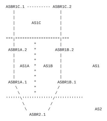
In the above figure, member-AS AS1A, AS1B, AS1C belong to a confederation of ASs in AS1. AS1A and AS1B are connected to AS2.
