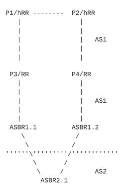
When the session between ASBR1.1 and ASBR2.1 undergoes maintenance, it is required that all BGP routers of AS1 reroute traffic to ASBR1.2 before the session between ASBR1.1 and ASBR2.1 is shut down.
