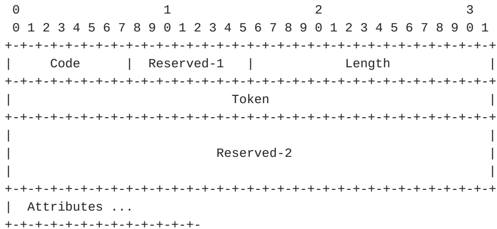
Figure 2: The RADIUS/1.1 Packet Format
