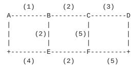
Node A is Ingress, Node D is Egress. A synchronized path computation requests for SRLG disjoint path may be issued using the SVEC object as described in [RFC5440]. In above topology a full SRLG disjoint paths are not possible because of some topology considerations.
