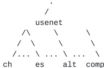
The structure described above, was supported by a faked root-server being the primary server for 'usenet.', and some secondary name servers for the same domain. Around a dozen collaborators participated in a small pilot, operating primary name servers for each of the hierarchies involved in addition to providing secondary name service for the 'usenet.' root zone.
