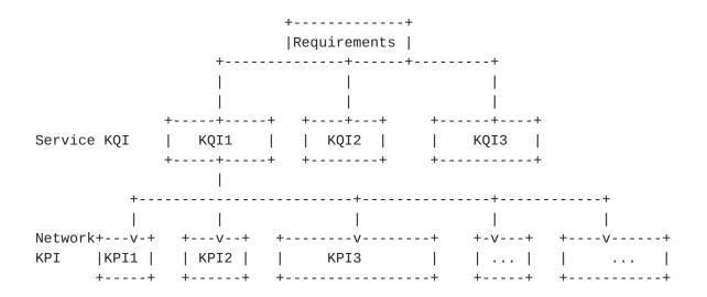
However, how to map URLLC and BAS application KQI to the corresponding set of network KPIs could be challenging. Furthermore, there could be potential need of defining new network KPI (e.g. latency down to 1ms must be provided with a reliability of 1-10^-9) to reflect some new application requirements.
