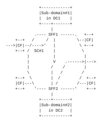
One path is shown from edge classifier to SFF1 to Sub-domain#1 to SFF1 to SFF2 to Sub-domain#2 to SFF2 to network eqress.
