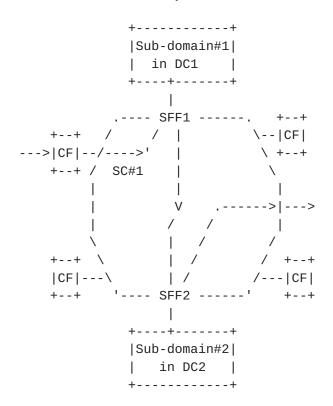
One path is shown from edge classifier to SFF1 to Sub-domain#1 (residing in data-center1) to SFF1 to SFF2 (residing in data-center 2) to Sub-domain#2 to SFF2 to network egress.
