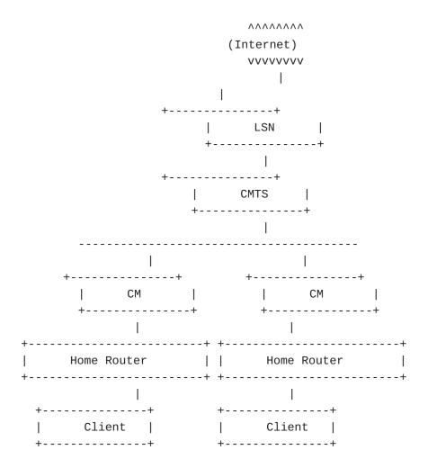
In this scenario, the two clients are under the same LSN but behind two different gateways. This simulates connectivity between two residential subscribers on the same ISP. We tested peer-to-peer applications. utorrent leeching and limewire leeching passed, while utorrent seeding and limewire seeding failed.
