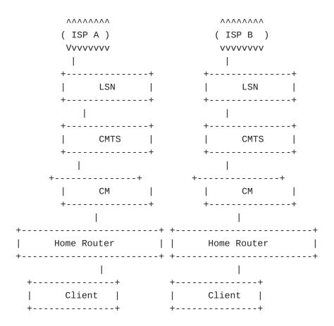
This test case is similar to Case 1 but with the addition of another identical ISP. This topology allows us to test traffic between two residential customers connected across the Internet. We focused on client-to-client applications such as IM and peer-to-peer. Instant messaging applications including Skype and Google Talk perform well. Skype video and voice chat also performed well. However, FTP transfers and peer-to-peer seeding failed.
