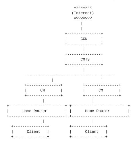
In this scenario, the two clients are under the same LSN but behind two different gateways. This simulates connectivity between two residential subscribers on the same ISP. We tested peer-to-peer applications.
