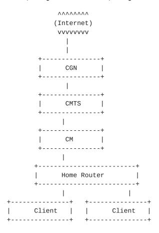
This is similar to Case 1, except that two clients are behind the same LSN and in the same home network. This test case was conducted to observe any change in speed in basic web browsing and video streaming.
