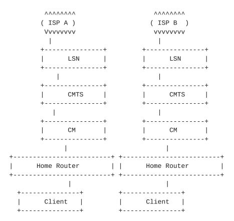
This test case is similar to Case 1 but with the addition of another identical ISP. This topology allows us to test traffic between two residential customers connected across the Internet. We focused on client-to-client applications such as IM and peer-to-peer.
