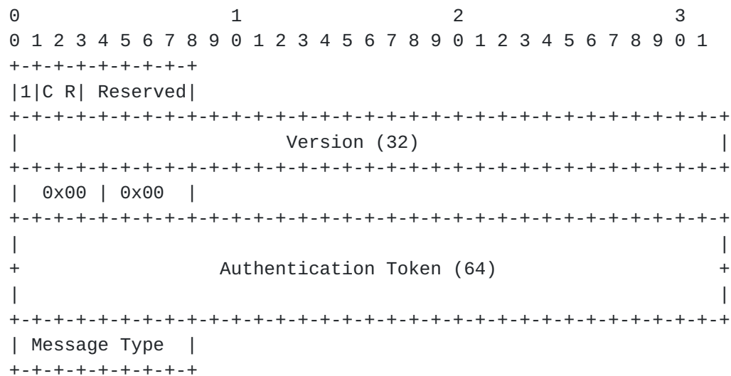
Figure 1: QUIC-LB Packet Format
