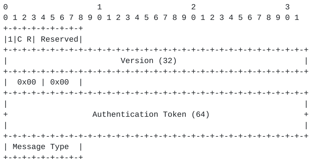
Figure 2: QUIC-LB Packet Format
