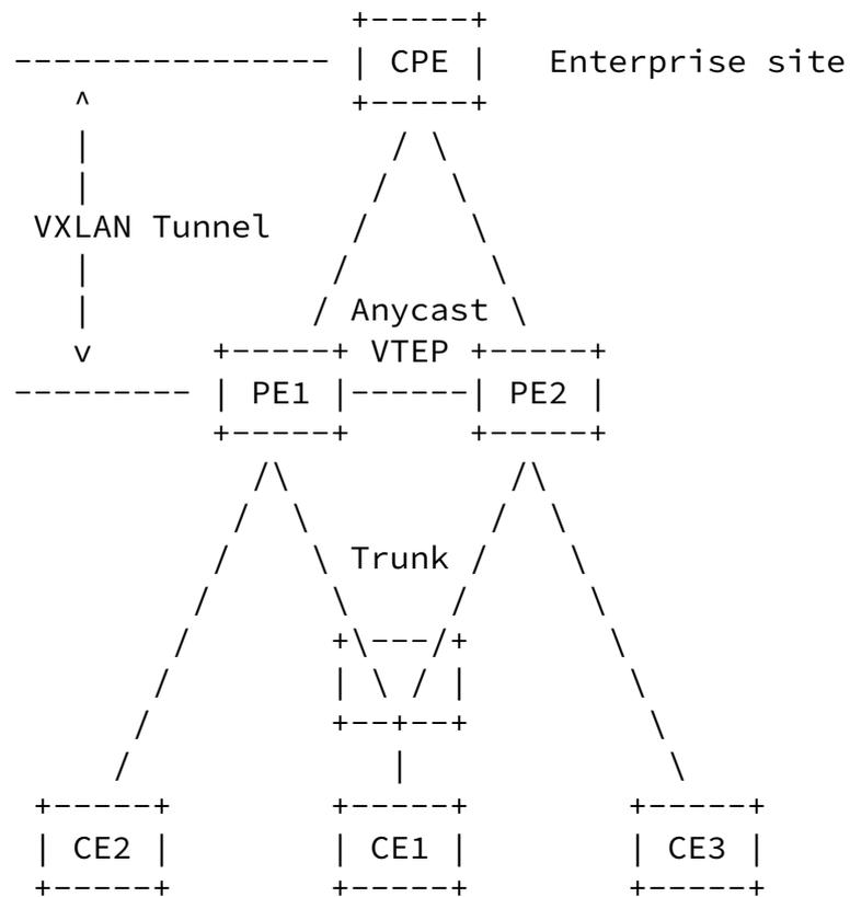
Figure 3. Basic networking of the VXLAN active-active scenario
