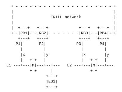
Further assume L1 and L2 are each bridged LANs that include a device M which maps VLAN-x into VLAN-y and VLAN-y into VLAN-x and that Fine Grained Labels [RFC7172] are not in use in the campus.
