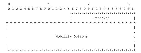
The Mobility Options field must always contain a Nonce option. The nonce must be stored locally by the CN for that MN, along with the address being tested. The nonce will be compared with the content of the nonce option found in the AOTR message.
