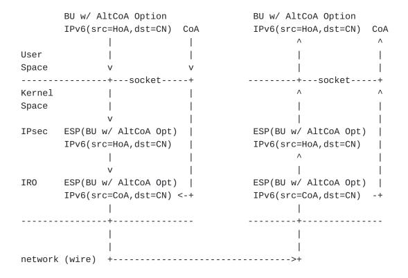
When the IPsec protected BU hits the remote MN, it passes the set of MIPv6 rules for the CN. It matches rule 2 so that its source address is remapped to the source address of the SA (the HoA of the MN). The source address found in the packet is stored as ancillary data. The packet is handled by the IPsec module, matches the SA, is decrypted and passed to the upper layer, the MIPv6 process.
