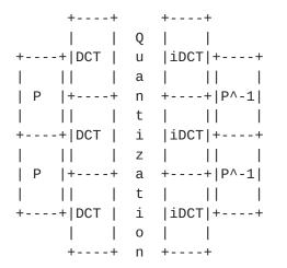
The pre-filter P operates in the time domain, processing block boundaries and removing inter-block correlation. The blocks are then transformed by the DCT into the frequency domain, where the resulting coefficients are quantized and encoded. When decoding, the inverse operator  $P^{-1}$  is applied as a post-filter to the output of the inverse DCT. This has two benefits:
