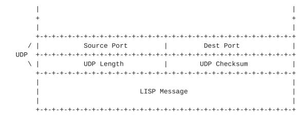
The LISP UDP-based messages are the Map-Request and Map-Reply messages. When a UDP Map-Request is sent, the UDP source port is chosen by the sender and the destination UDP port number is set to 4342. When a UDP Map-Reply is sent, the source UDP port number is set to 4342 and the destination UDP port number is copied from the source port of either the Map-Request of the invoking data packet.
