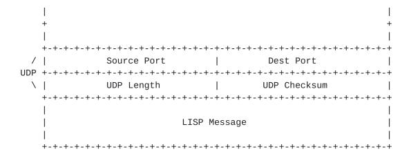
The LISP UDP-based messages are the Map-Request and Map-Reply messages. When a UDP Map-Request is sent, the UDP source port is chosen by the sender and the destination UDP port number is set to 4342. When a UDP Map-Reply is sent, the source UDP port number is set to 4342 and the destination UDP port number is copied from the source port of either the Map-Request or the invoking data packet.
