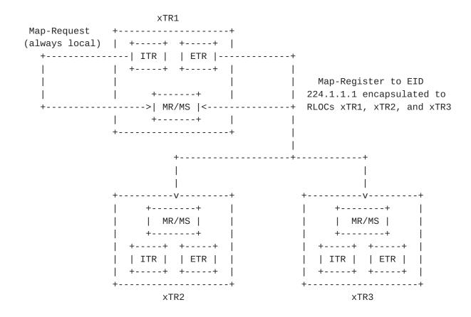
Note if any external xTR would like to use a Map-Resolver from the mapping system group, it only needs to have one of the LISP-Decent Map-Resolvers configured. By doing a looking to this Map-Resolver for EID 224.1.1,1, the external xTR could get the complete list of members for the mapping system group.
