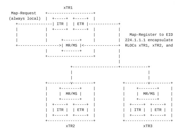
Note if any external xTR would like to use a Map-Resolver from the mapping system group, it only needs to have one of the LISP-Decent Map-Resolvers configured. By doing a looking to this Map-Resolver for EID 224.1.1,1, the external xTR could get the complete list of members for the mapping system group.
