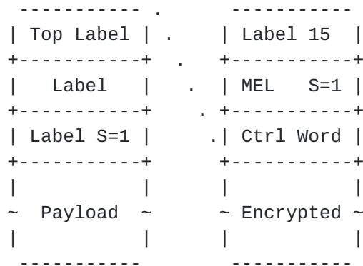
Figure 1 : The Use of the MEL for Hop-by-Hop Encryption
