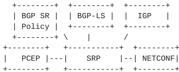
Figure 2: Topology/link-state database architecture
