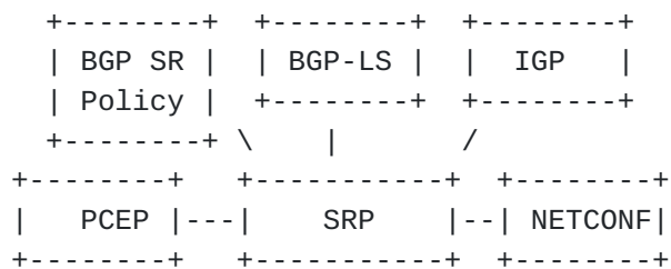
Figure 2: Topology/link-state database architecture
