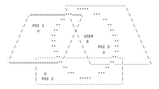
Figure 3: LoST client location (circle) overlapping three service areas of three different points of interest (POI 1, POI 2, POI 3)
