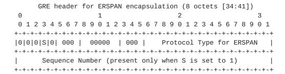
Note that in the above GRE header [RFC1701] out of the C, R, K, S, s, Recur, Flags, Version fields only S (bit 03) may be set to 1. The other fields are always set to zero.
