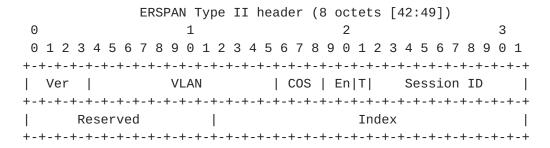
The above 8-octet header is immediately followed by the original mirrored frame and then by the standard 4-octet Ethernet CRC:
