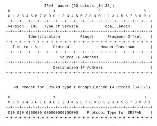
This encapsulation adds 38 octets to the original frame length: 14 (MAC) + 20 (IP) + 4(GRE). The advantage of this format is its size, which is more compact than Type II's and therefore can be less expensive to implement.
