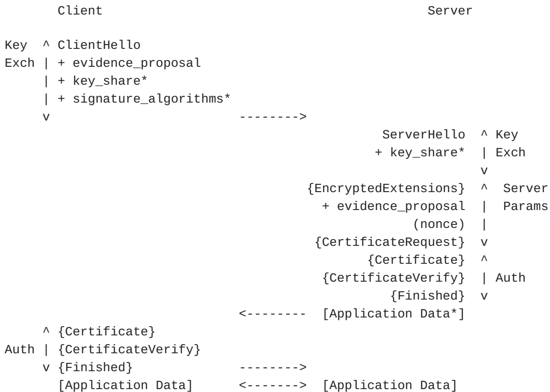
Figure 1: TLS Client Providing Evidence to TLS Server.
