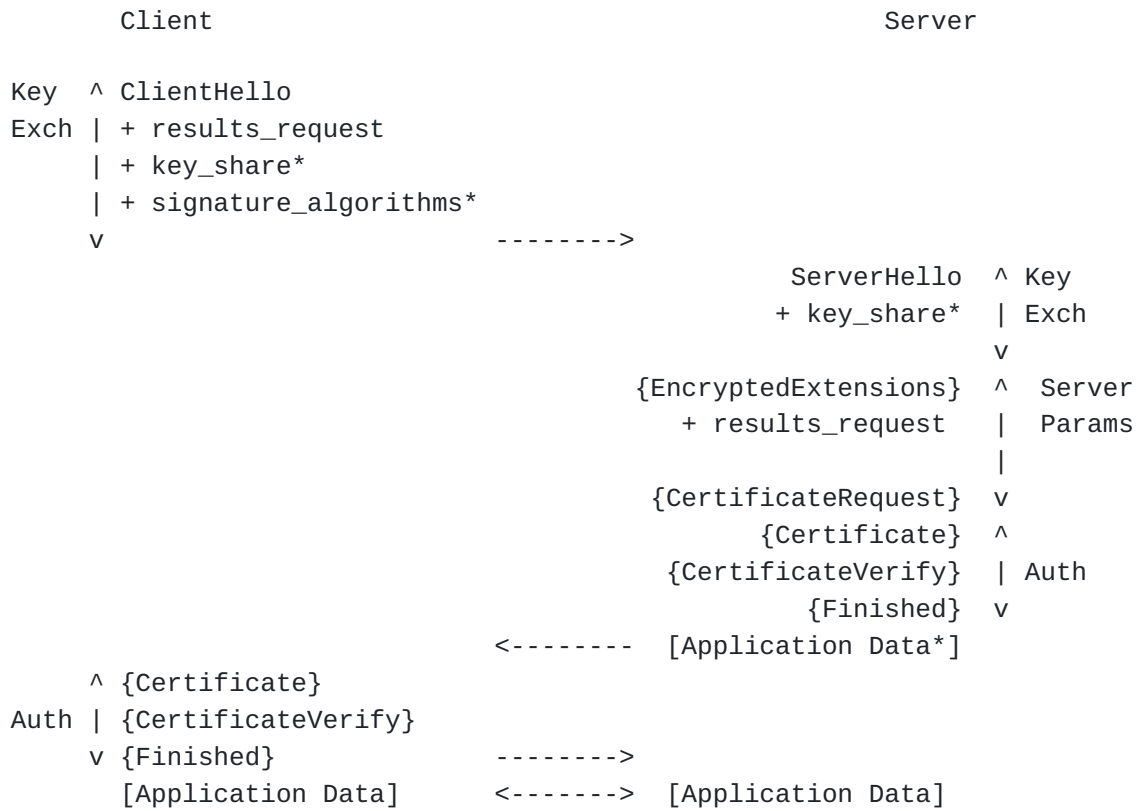
Figure 4: TLS Server Providing Attestation Results to TLS Client.
