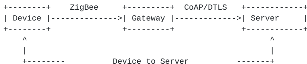
Figure 1: IoT Closed Network Gateway
