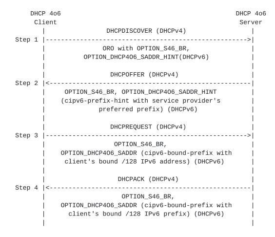
IPv6/IPv4 Binding Message Flow
