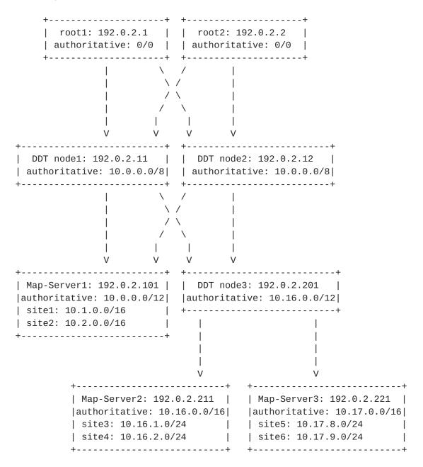
DDT nodes are configured for this "root" at IP addresses 192.0.2.1 and 192.0.2.2. DDT Map Resolvers are configured with default referral cache entries to these addresses.
