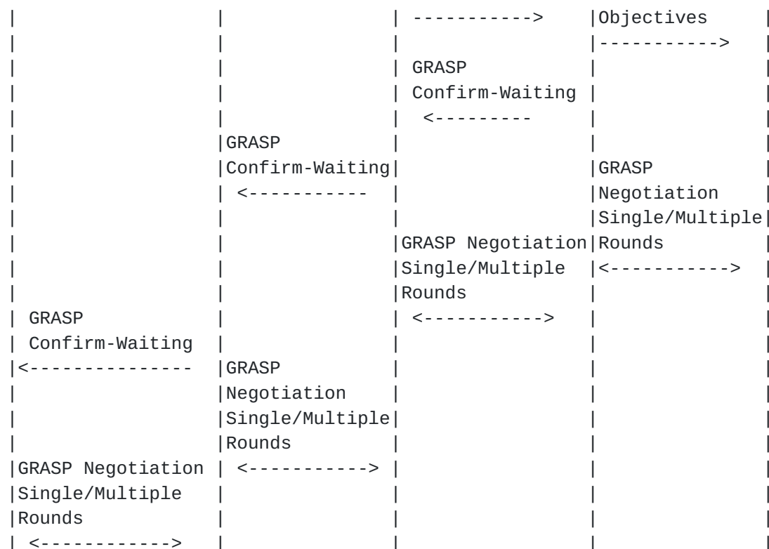
Figure 2 - GRASP: Network Slice reservation / Release3 Messages Flow
