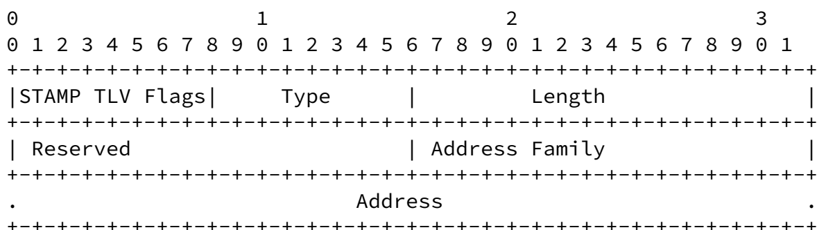
Figure 4: Return Address Sub-TLV in Return Path TLV
