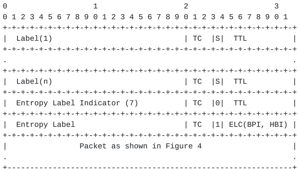
Figure 5: Example MPLS Encapsulation for IOAM using BOS Header
