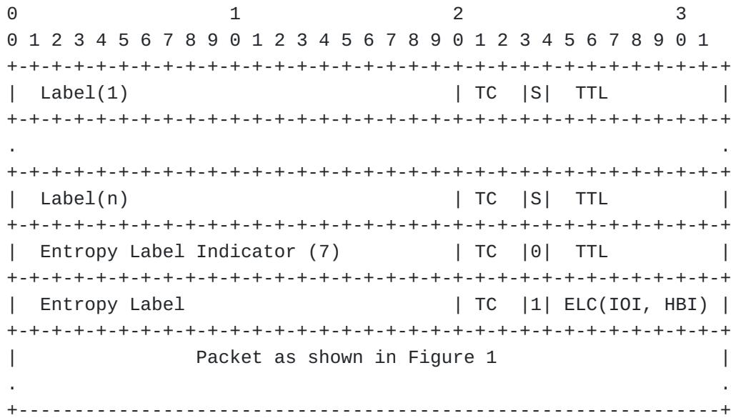
Figure 3: Example MPLS Encapsulation for HBH IOAM
