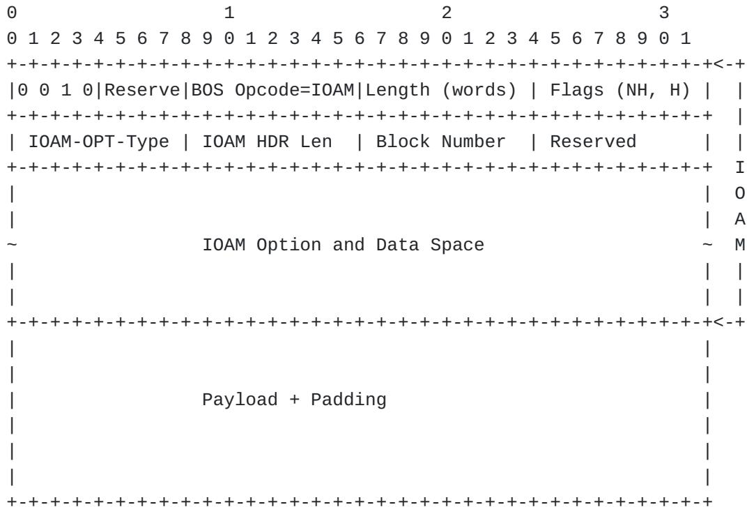
Figure 4: IOAM BOS Extended Header with IOAM Data Fields
