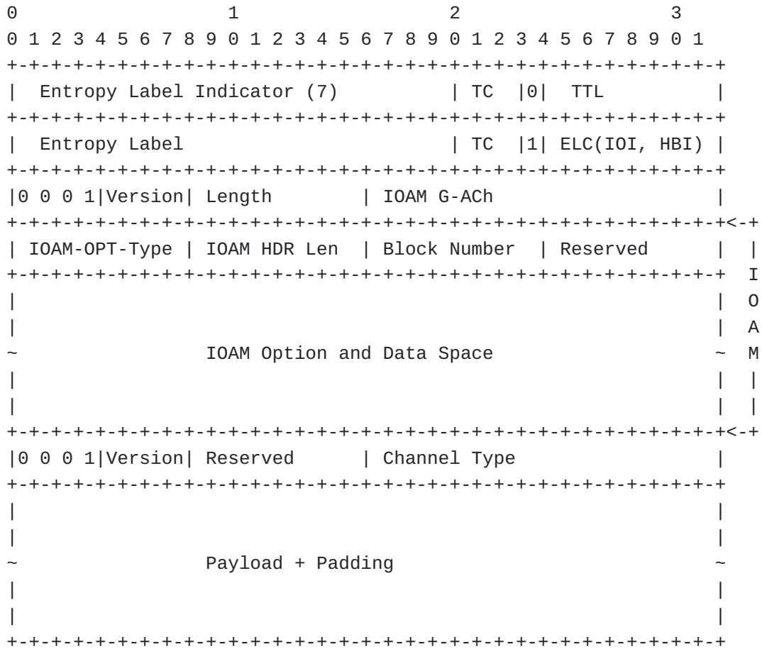
Figure 7: Example MPLS Encapsulation with Another G-Ach with HBH IOAM
