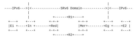
As the figure shows, an IPv6 flow is sent out from the end station E1. The packet of the flow is encapsulated in an outer IPv6+SRH header in the Ingress(In) and transported through an SRv6 domain. In the Egress(Eg), the outer IPv6+SRH header of packet is popped, and the packet is sent to the destination E2.
