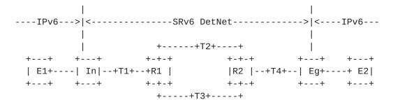
The figure above shows that an IPv6 flow is sent our from the end station: E1. The packet of the flow is encapsulated as a DetNet SRv6 packet in the Ingress(In) and transported through an SRv6 DetNet domain. In the Egress(Eg), the upper IPv6 header with SRH of the packet is popped, and the packet is transmitted to the destination(E2).
