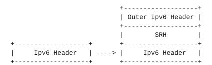
The outer IPv6 Header with SRH is used for carrying DetNet flows. Traffic Engineering is programmed in the segment list of SRH, and other functions and arguments for service protection (packet replication, elimination and ordering) and congestion control (packet queuing and forwarding) are also defined in SRH.
