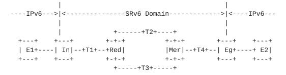
As the figure shows, an IPv6 flow is sent out from the end station E1. The packet of the flow is encapsulated in an outer IPv6+SRH header in the Ingress(In) and transported through an SRv6 domain. In the Egress(Eg), the outer IPv6 header+SR of the packet is popped, and the packet is sent to the destination E2.
