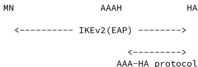
Figure 2 - Dynamic MIPv6 bootstrapping through IKEv2 and EAP
