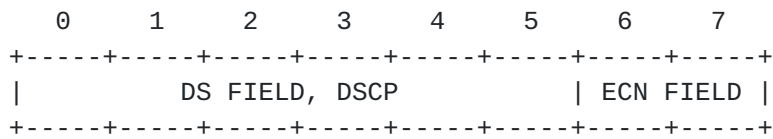
Figure 6: The Differentiated Services and ECN fields in IP
