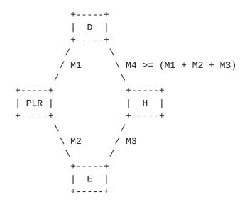
The protection router (PLR) evaluates for a primary path to destination 'D' if  $\{E \rightarrow H \rightarrow D\}$  is a viable backup path. Because the metric M4  $\{H \rightarrow D\}$  is higher than the sum of the original primary path and the path from router 'H' to the PLR, this particular path would result in a loop and therefore is rejected.
