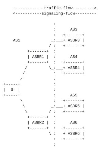
ASBR {1,2} may want to periodically check the liveliness state to the endpoint of the label (ASBR {3,4,5,6}) which they are advertising. BFD Echo mode [<u>RFC5880</u>] is suitable technology to ensure liveliness state of undirectional links.
