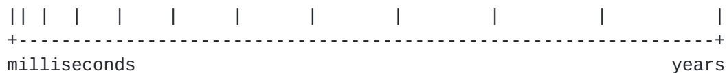
Figure 1: A logarithmic range representation allows for higher precision in the smaller time ranges and still supports large time deltas.
